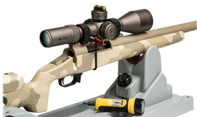
Using bubble levels to square the riflescope to the base.
