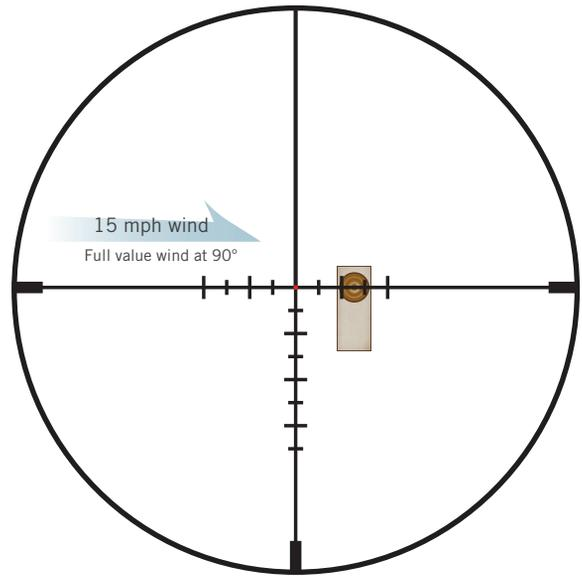
2.6 mrad reticle correction for 15 mph wind at 600 yards. Elevation is already dialed into turret.
