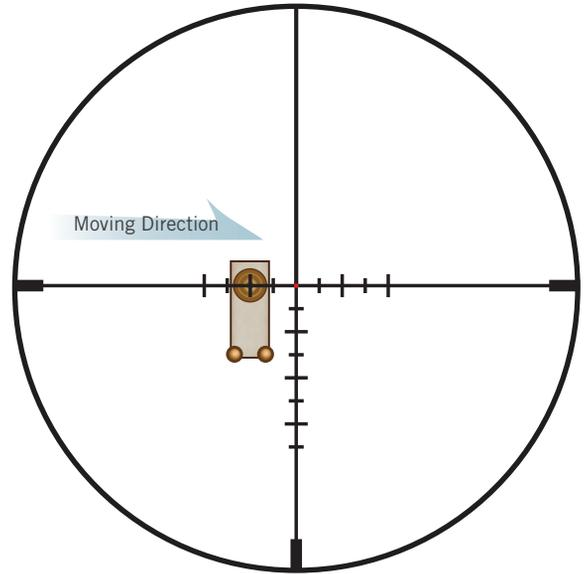
2 mrad reticle correction for a target moving 3 mph at a distance of 600 yards. Elevation already dialed into turret.
